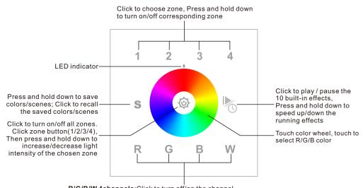
**R/G/B/W 4channels**:Click to turn off/on the channel Press and hold down to increase/decrease light intensity of each channel
